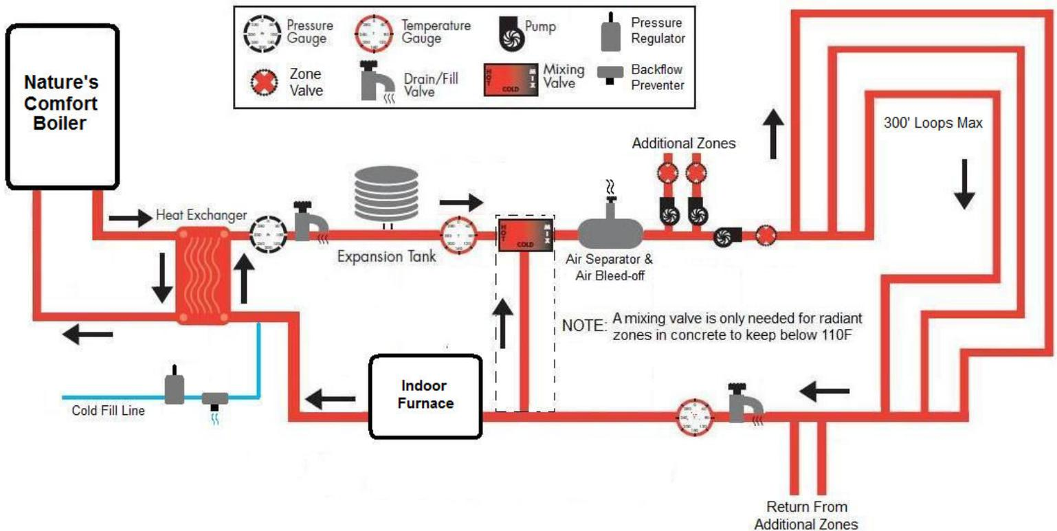
As shown in the previous drawing, the two systems are totally isolated from each other so that the existing hydronic system remains undisturbed and functions exactly as it did before. Water that circulates through the outdoor boiler is never circulated through the home's hydronic system or vice-versa.
