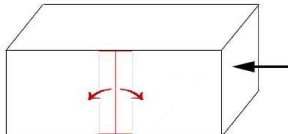
Bend the sheet metal back and out, along the grey lines.
