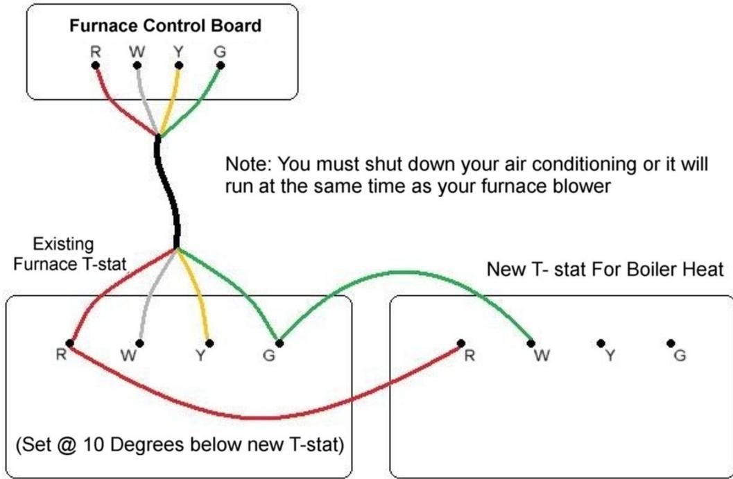
Use the example drawing below if you have a 2 wire system, don't have a blower-only function or the thermostat is the advanced computerized type that communicates back and forth between the furnace (typically found on heat pump systems). **Do not use this method if your HVAC system utilizes a multi-speed blower.** All of the parts below are available through Nature's Comfort.
