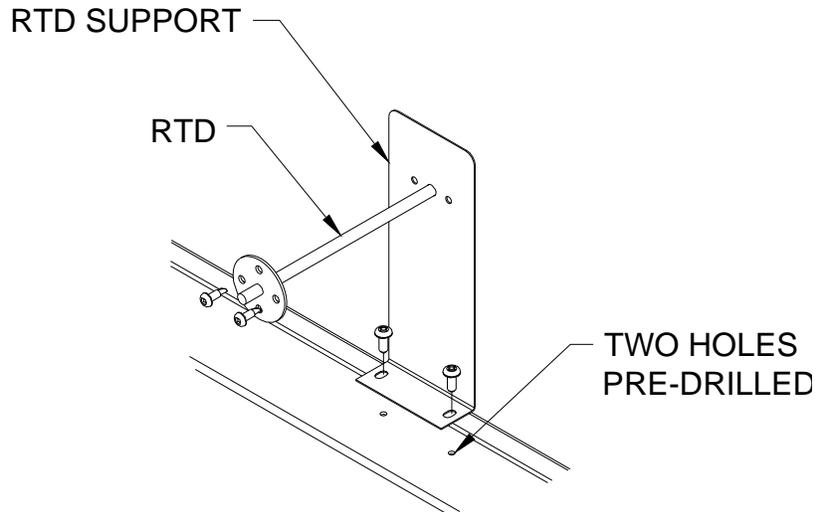
It is important that the RTD and the RTD support be properly fixed onto the plenum.
