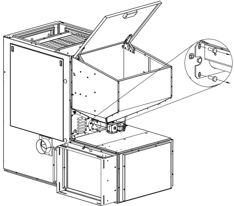
3- Loosen the screws inside the hopper. Lift it and pull it backwards.
