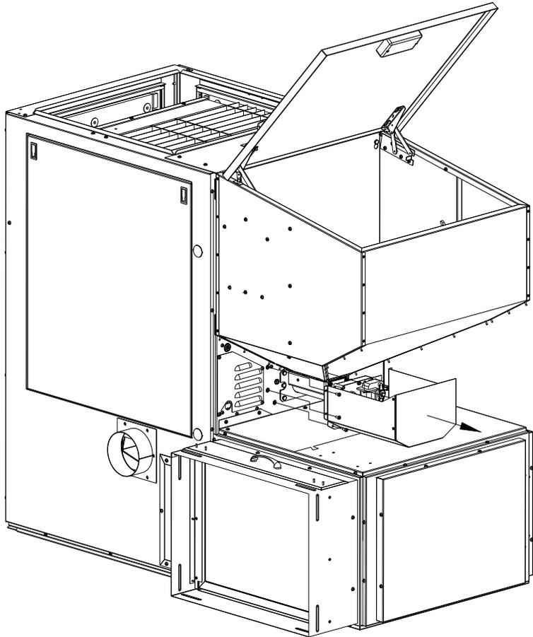
2- Remove the screws from the hopper support (keep the screws).
