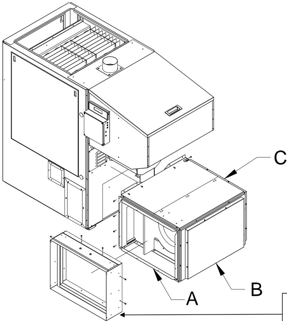
The cold air ducting support is not installed on the blower assembly. It can be installed as per configurations A, B, or C. It is supplied in the hopper.
