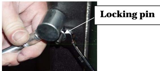
2. To increase the pressure of the door on the gasket, turn the handle counter clockwise; to decrease the pressure of the door on the gasket, turn the handle clockwise until desired pressure is attained.
