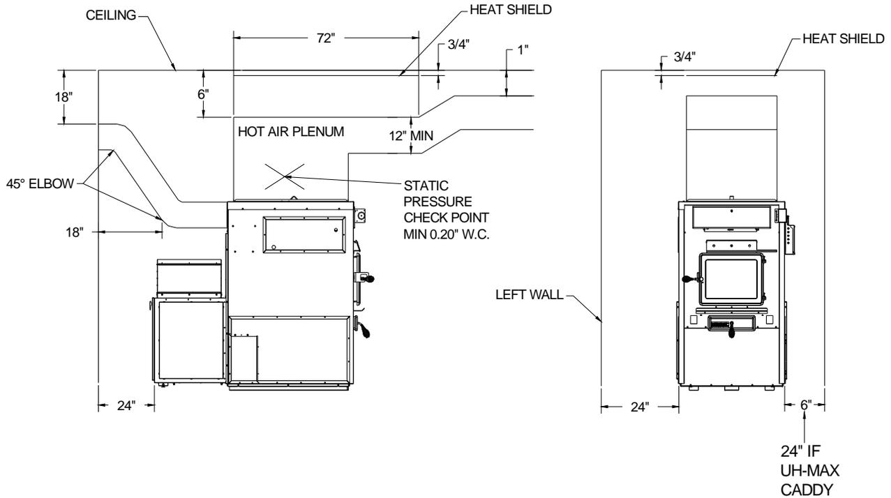
**N.B. THE SIZE OF THE AIR RETURN DUCT SHOULD BE AT LEAST EQUAL TO THE SIZE OF THE COLD AIR PLENUM OPENING.**
